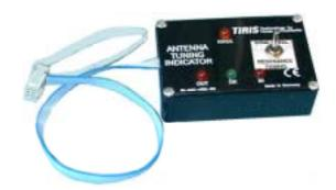
The Antenna Tuning Indicator makes the resonance tuning of TI-RFid's Standard RFM (RI-RFM-104B) and the High Performance RFM (RI-RFM-007B) easy. LED's indicate in which direction the tuning core should be turned (RI-RFM-104B) or whether tuning capacitance need to be added or removed (RI-RFM-007B) to bring a connected antenna to resonance.
